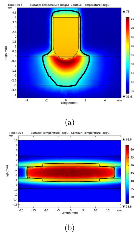
Fig. 5. Diagrams of thermal field spreading in time: monopolar electrode (a), bipolar electrode (b)
