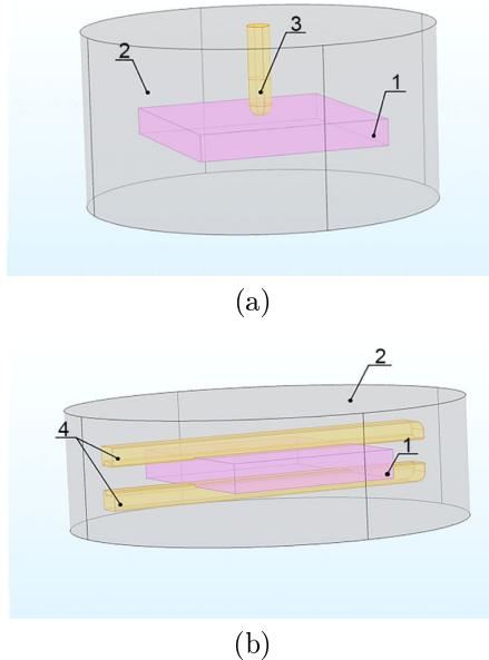
Fig. 4. Geometry of mathematical models for monopolar (a) and bipolar (b) ablation, where 1 – is the myocardium tissue, 2 – is the ambient air, 3 – is the monopolar electrode, 4 – is clamps of the bipolar electrode
