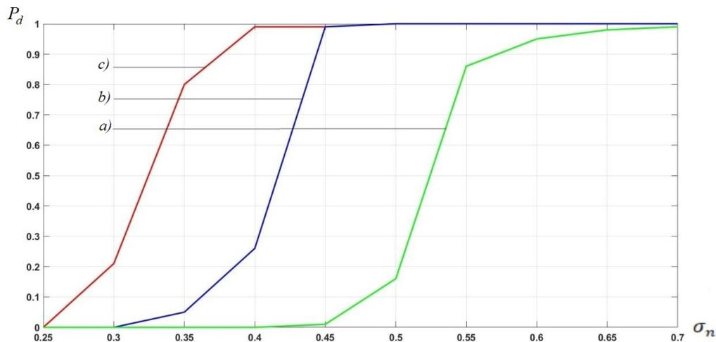
Fig. 7. Tracking failure probabilities for images a) 25 by 15, b) 18 by 12, c) 10 by 6 pixels
