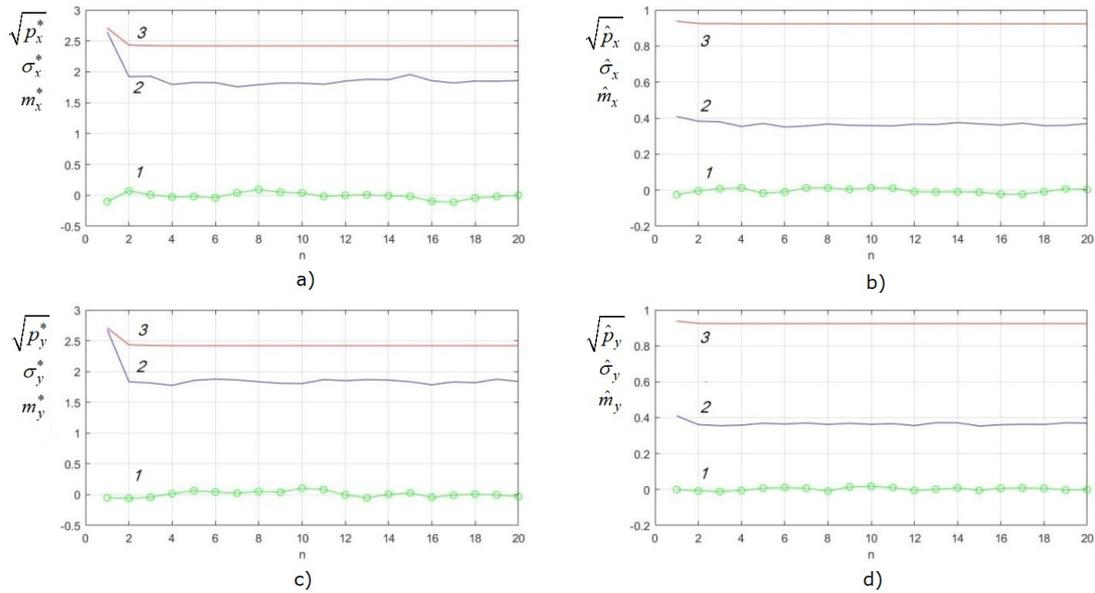
Fig. 6. Dependences of mathematical expectation and SD of forecast errors and estimates UAV coordinates on the X and Y axes
