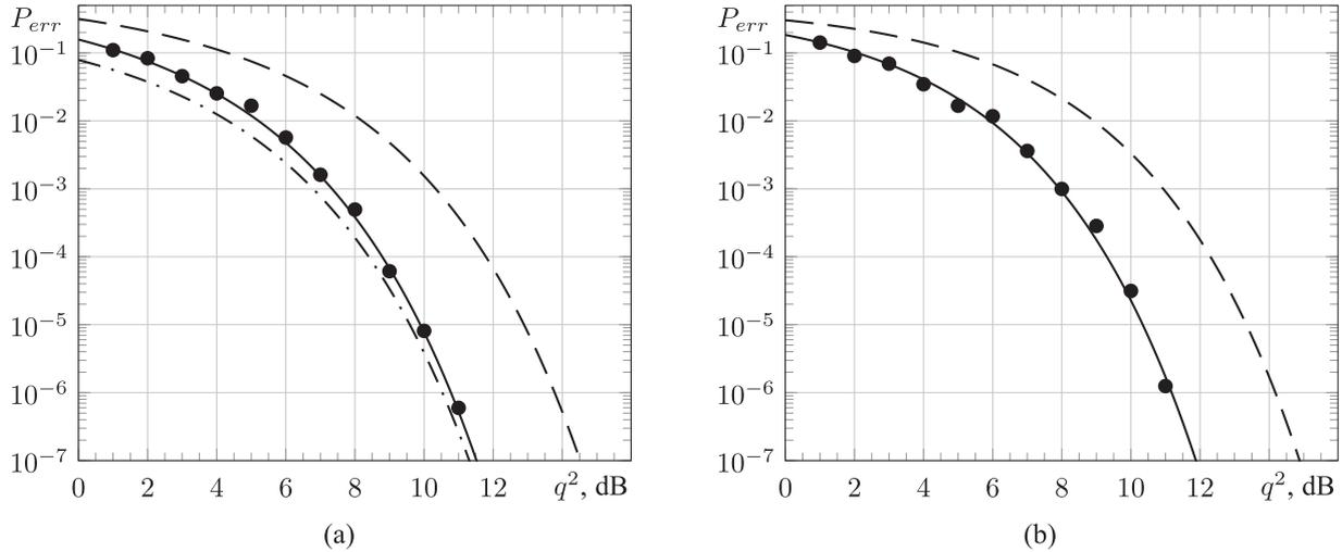
Fig. 5. Curves of potential noise immunity of coherent (a) and incoherent (b) reception of BPSK signals with Manchester encoding and DBPSK signals with differential Manchester encoding
