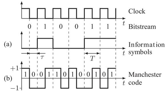
Fig. 1. Bitstream encoding by the Manchester code
