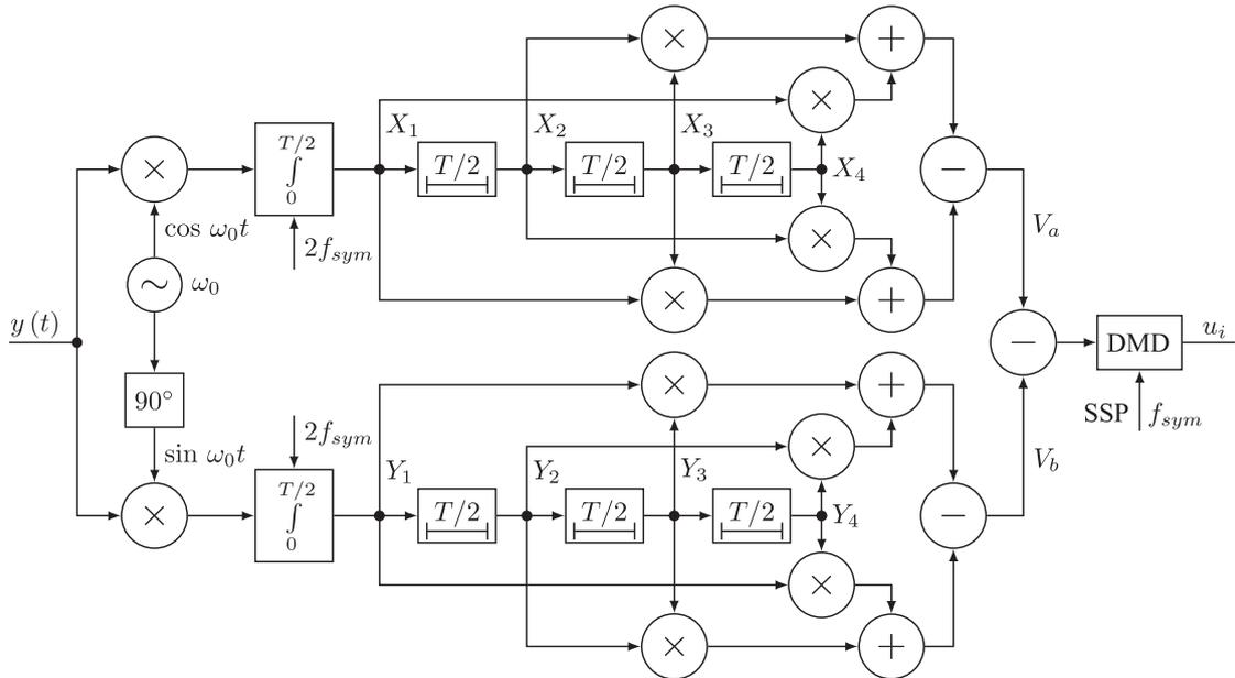
Fig. 4. Block diagram of the optimum incoherent demodulator of DBPSK signals with differential Manchester encoding
