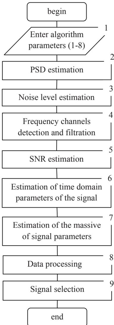
Fig. 1. Block diagram of signal selection algorithm
