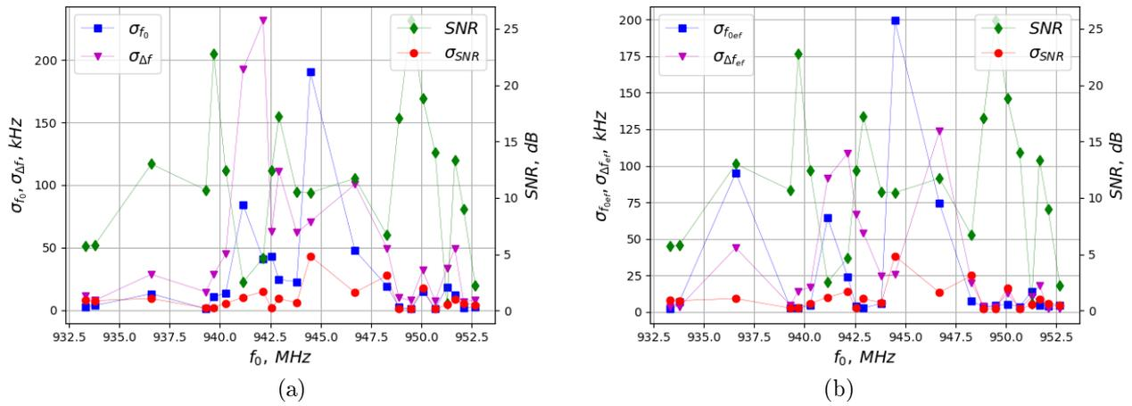
Fig. 8. Dependences of  $\sigma_{f_0}$ ,  $\sigma_{\Delta f}$ , SNR,  $\sigma_{SNR}$  estimates on center frequency (a) and a similar graph for  $f_0$ ,  $\Delta f$  SD estimates, obtained by expressions (4) and (5) (b)
