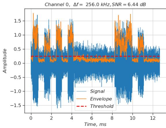
Fig. 6. Time domain signal processing for channel No. 0
