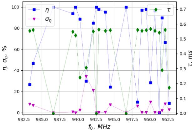
Fig. 10. Dependence of  $\eta$ ,  $\sigma_\eta$ ,  $\tau$  estimates on center frequency
