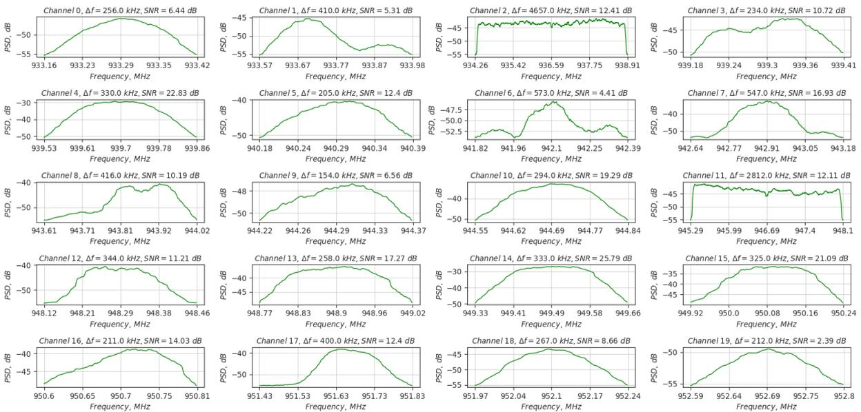
Fig. 4. PSD for each frequency channel after additional smoothing
