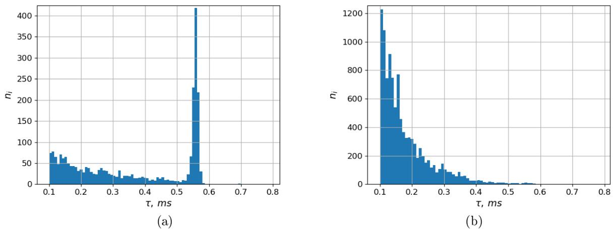
Fig. 9. Histograms of measured pulse durations in channel No. 0 (a) and No. 19 (b)
