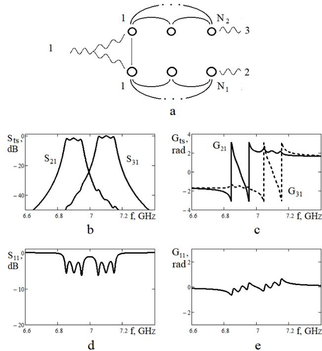
Fig. 6. Demultiplexer built on 3+3 different DR (a). Scattering characteristics of the detuned in frequency 2 bandpass filters ( $f_1 = 6,9$  GHz;  $f_2 = 7,1$  GHz;  $Q^D = 2 \cdot 10^3$ ; coupling coefficients of resonators with the line:  $k_L = 0,006$ ; mutual coupling coefficients of adjacent filter resonators:  $k_{12} = 0,01$ ; mutual coupling coefficients of input 1-1 resonators (a):  $k^{FF} = 0,005$ )
