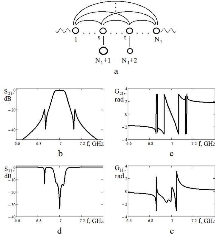
Fig. 5. Elliptical bandpass filter on 3+1+1 different DRs in a transmission line break (a). Scattering characteristics of the filter ( $f_1 = 7$  GHz;  $f_2 = 6,87$  GHz;  $f_3 = 7,13$  GHz;  $Q^D = 2 \cdot 10^3$ ; coupling coefficients of resonators with the line:  $\tilde{k}_L = 0,012$ ; mutual coupling coefficients of adjacent filter resonators:  $k_{12} = 0,011$ ; mutual coupling coefficients of line resonators and shunt resonators:  $k^F = 0,01$ ;  $s = 1$ ;  $t = 3$ )
