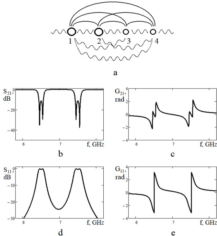
Fig. 2. 2+2 different DR system in a transmission line (a). Scattering characteristics of two different bandstop filters in the transmission line ( $f_1 = 6,5$  GHz;  $f_2 = 7,5$  GHz;  $Q^D = 2 \cdot 10^3$ ;  $\Gamma\Delta z_{12} = \pi/2$ ; distance between extreme filter resonators  $\Gamma\Delta z_F = 2\pi$ ; coupling coefficients of resonators with the line  $\tilde{k}_L = 0,015$ ; mutual coupling coefficients of adjacent resonators  $k_{12} = 0,005$ )
