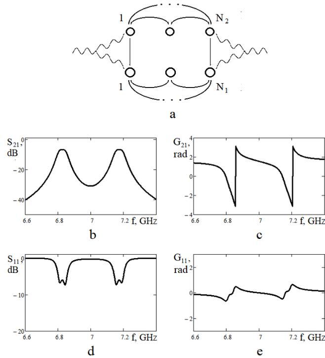
Fig. 3. 2+2 different DR system in a transmission line break (a). Scattering characteristics of two parallel bandpass filters ( $f_1 = 6,85$  GHz;  $f_2 = 7,15$  GHz;  $Q^D = 2 \cdot 10^3$ ; coupling coefficients of resonators with the line:  $k_L = 0,006$ ; mutual coupling coefficients of adjacent filter resonators:  $k_{12} = 0,006$ ; mutual coupling coefficients of input (output) resonators:  $k^F = -0,025$ )
